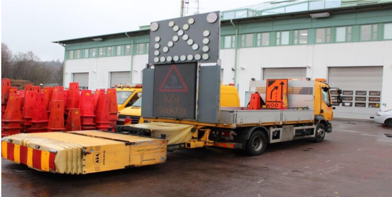
Road Works Vehicle with Truck Mounted Attenuator (TMA)
