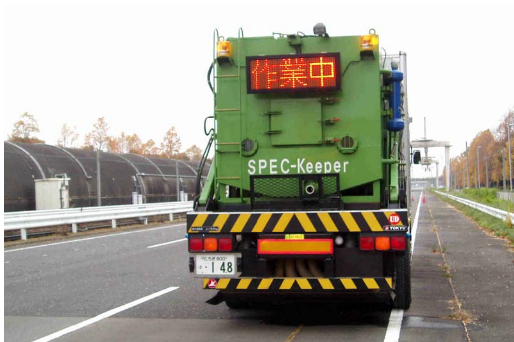
Figure 9. Cleaning machine using high pressure water.
