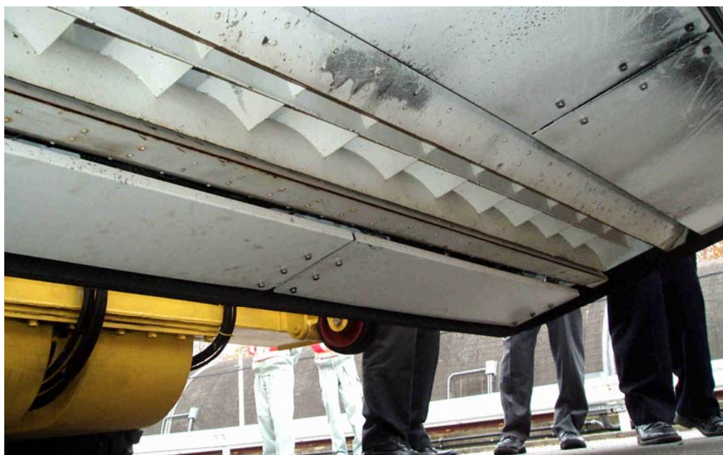
Figure 11. Inside the enclosure where the high pressure air cleaning is performed
