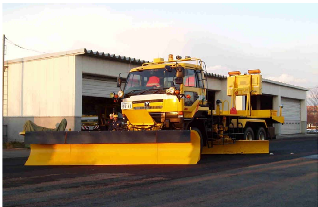
Figure 31. Heavy snow moving material with steel plough used in the Hokkaido road districts.
