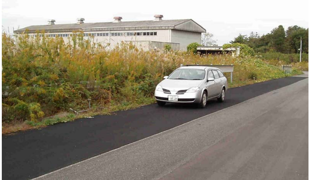
Figure 12. Test section with porous elastic pavement at the PWRI test track. The noise from a passenger car passing was very low and the high frequencies from air pumping noise were reduced significantly.
