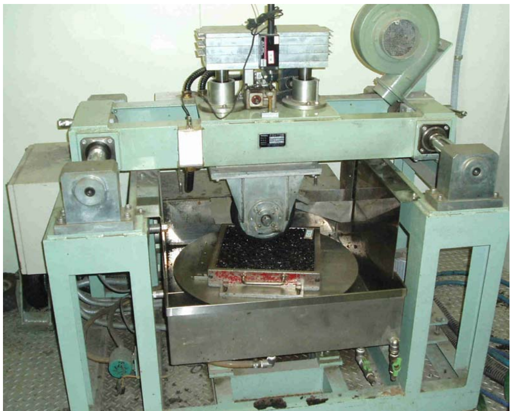
Figure 16. The rotating pavement durability tester.
