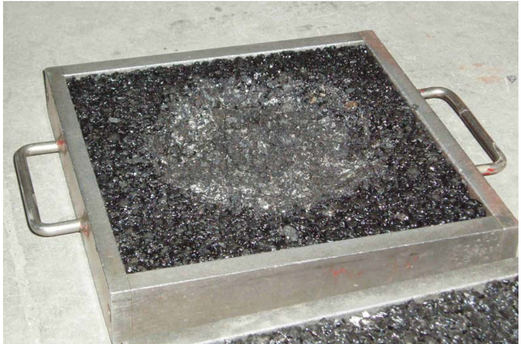
Figure 17. Pavement slaps produced at the laboratory after it is tested in the wheel tracking device.
