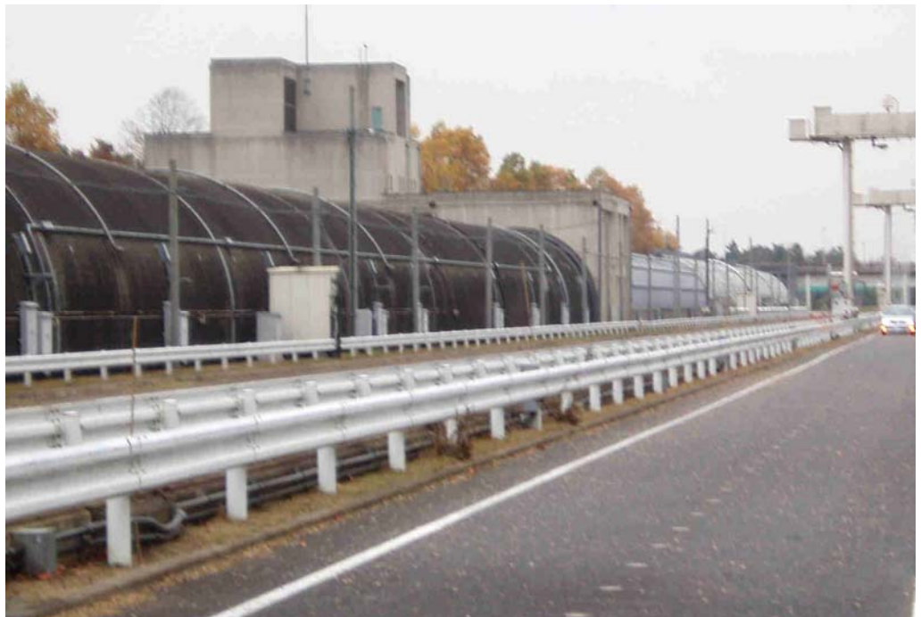
Figure 4. The PWRI test tunnel. Testing of warning systems for wind and severe meteorological conditions and research into visibility of road markings.
