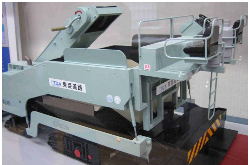
Figure 20. Model of the Muti-Asphalt Layer Machine (MAP) that can apply two layer pavements in a warm in warm process.
