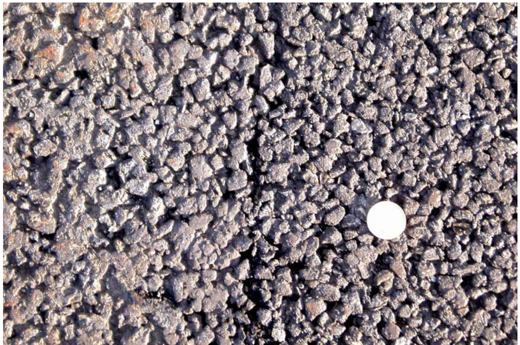
Figure 35. Close up of the porous (to the right) and the hybrid pavements both with 13 mm aggregate.
