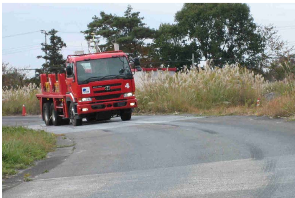
Figure 5. The circle test track at PWRI and an automatic controlled three axels heavy truck without driver.
