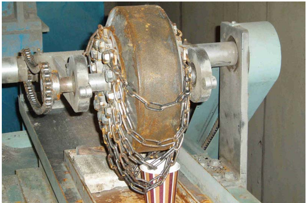
Figure 18. Durability tester with steel chains mounted on the wheel in order to simulate the effect of raveling from snow chains in cold regions. This test is performed at minus 10 °C.
