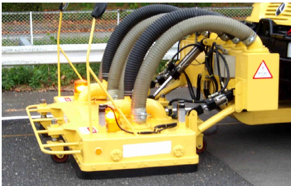
Figure 10. Cleaning machine using high pressure air.
