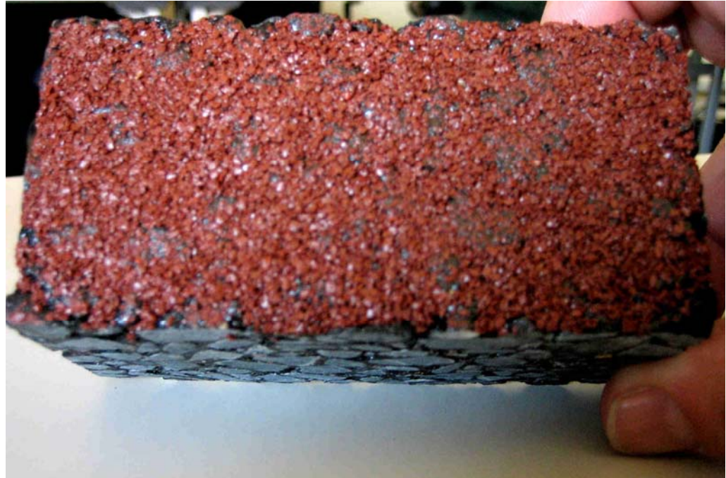
Figure 22. Read version of Permeable Resin Mortar System (PERMS) is a resin mortar with fine (porous) ceramic material (aggregate size 1.5 mm) that is applied as a surface treatment on porous pavement.
