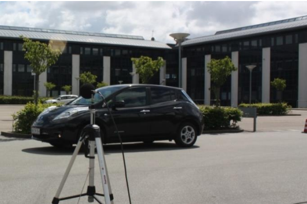
Figure 4 Microphone setup with part of a traffic cones to the right and the Nissan Leaf passing the microphone.
