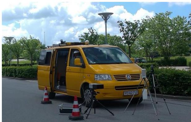
Figure 2: Photo of the measurement operative vehicle. In the center speed is measured with a laser to the right the air temperature is measured. The mount furthest to the right was used to record some measurements on film.
