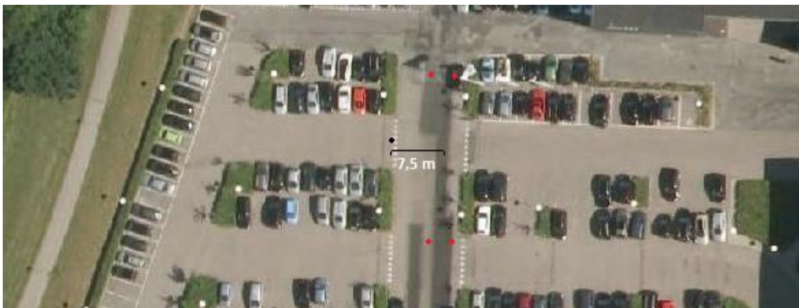
Figure 1 Photo for the CPB test site from the summer 2012, before it was repaved. The red dots symbolize the traffic cones confining the measuring zone. The black dot symbolizes the microphone, which is 7.5 m from the center of the test lane.
