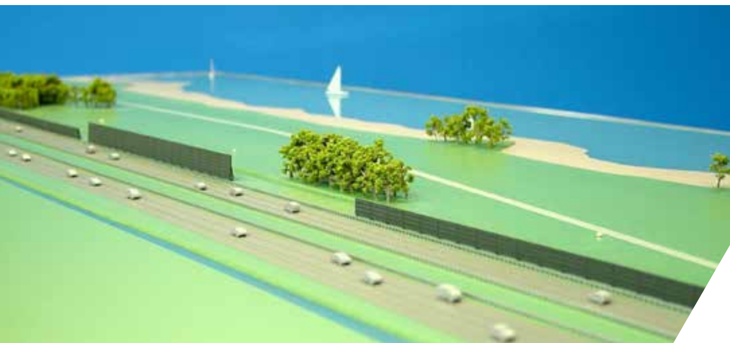
FIGURE 15. The model of the IPL test location between a beach and a highway. This shows three different types of noise barrier. Image reprinted with acknowledgement from Rijkswaterstaat Centre for Transport and Navigation and M+P, see ref. 46.
