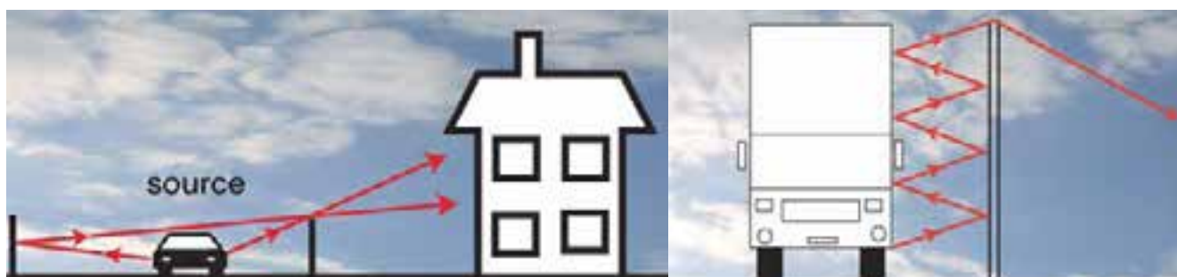
FIGURE 2. Left: Reflections between two parallel screens can increase the noise level on the adjacent side. Right: Multiple reflections between a high vehicle and a noise barrier can have similar consequences. In both examples absorbing material on the road side of the noise barrier may reduce the reflections. From ref.10, © 2009, reproduced by permission of Taylor & Francis Books UK.
